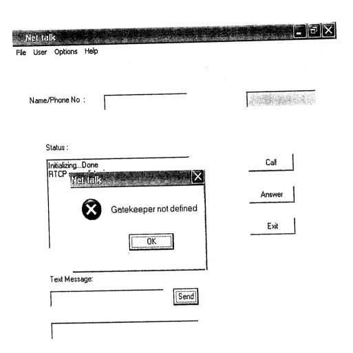
The client should connect to gatekeeper to advertise its presence. The gatekeeper should have static IP address, so that client defines the address of gatekeeper to establish connection. If gatekeeper address is not defined or invalid address is defined this error message instructs user to define valid gatekeeper address.
