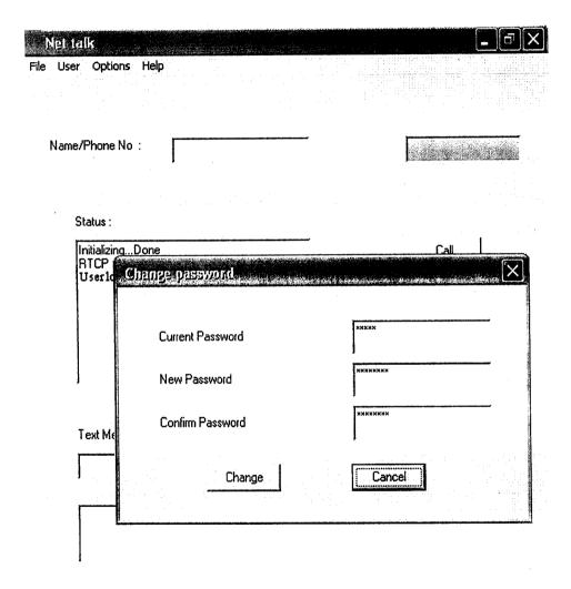
The user can change the password at any time. The user should first login, and should supply current password and new password (twice). The password details are sent to gatekeeper where the password is validated and if found valid the password is changed to new one.
