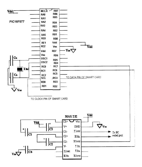
Selecting a FLASH PICmicro Microcontroller from the mid-range family as the target MCU allows us to make the code simpler and cleaner. It also provides larger RAM memory space and a deeper hardware stack. Interrupts have been used to "virtualize" the receiving routine as a software peripheral and to free the design of the hard real time constraint that it usually poses.
