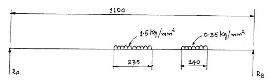
Reaction,  $R_A = 1.5 \times 235 \times 550 + 0.35 \times 140 \times 341/1100$  $R_A = 178 \text{ Kg}$
