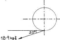
Vertical force acting on the shaft =  $18.9 \sin 20^{\circ}$
