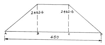
We know that the equivalent twising moment  $=\frac{\pi}{32}x$  f<sub>b(max)</sub>x d<sup>3</sup>
