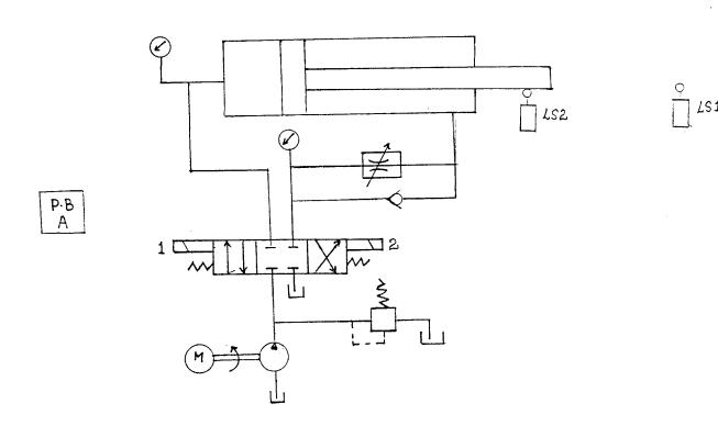
Pressing push button A, solenoid 1 of the directional Control Valve is activated, which allows the fluid to the cap end of the cylinder. The flow Control Valve installed in the rod end chamber of the cylinder line limits the fluid flow through it
