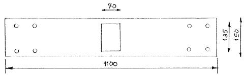
A section of dimension  $135 \times 70 \text{ mm}$  is cut from the top portion of the channel using a gas cutting machine along its depth to facilitate the belt movement.
