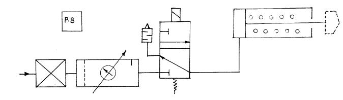
Pressing the push button A, the directional Control Valve is activated which makes the air flow from the power pack to the cap end of the cylinders.
