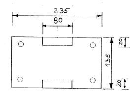
Using taps, threads are cut inside the holes for fixing the arbor with the main beam using bolts.
