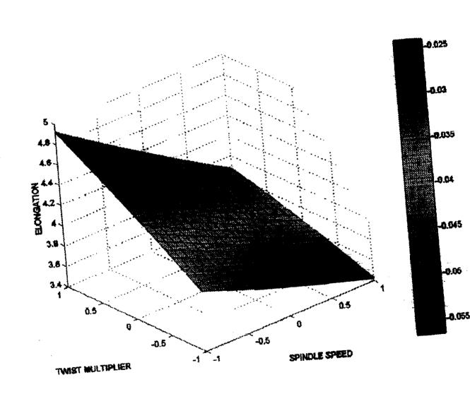
The effect of spindle speed and TM at a given traveler size of 6/O can be seen in the graph. It is observed that the yarn elongation value decreased gradually when the spindle speed is increased from 14000 to 16000 rpm. The change in yarn elongation was curvilinear when the TM is increased from 3.75 to change in yarn elongation was curvilinear when the TM is increased and TM 4.25. Thus for a given traveler number, the influence of spindle speed and TM
