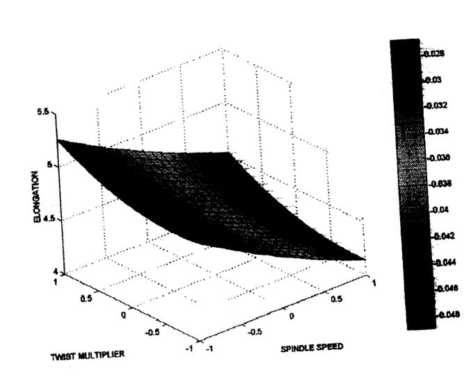
As per the graph at a given traveler number of 14/O, the yarn elongation abruptly decrease with increase in spindle speed from 14000 to 16000 rpm. The yarn elongation value increases almost linearly with increase in TM values between 3.9 and 4.3. The effect of spindle speed is much more pronounced than
