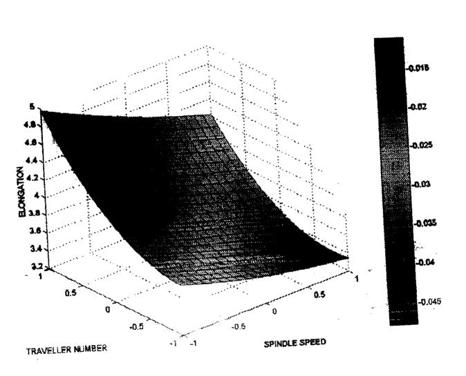
At a TM of 4.1, the yarn elongation was found to decrease with increasing spindle speeds from 14000 to 16000 rpm. The yarn elongation was found to increase with increasing traveler number from 10/O to 14/O. At this particular value of TM, the effect of traveler number was found to be lesser than that of
