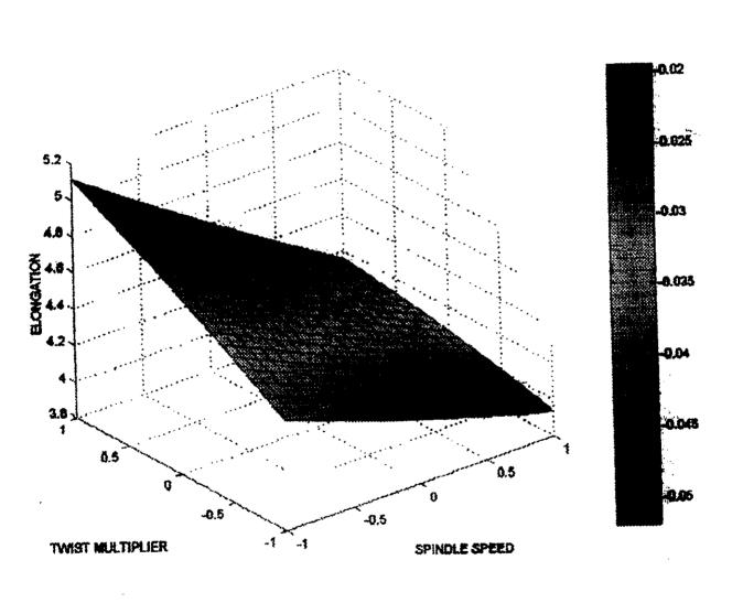
The effect of spindle speed and TM at a given traveler size of 7/O can be seen in the graph. It is observed that there is a drastical decrease in yarn elongation when spindle speed is increased from 14000 to 16000 rpm. The yarn elongation steadily increases with change in TM values from 3.75 to 4.25. Thus
