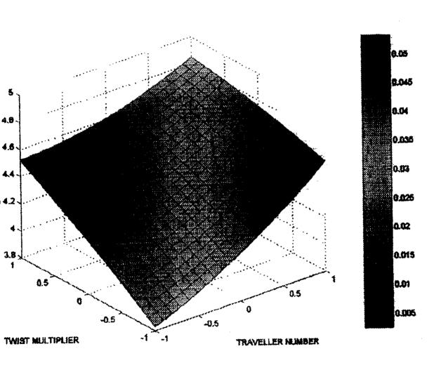
From the graph it can be observed that the yarn elongation increases sharply with increase in traveler number from 6/O to 8/O and TM values between 3.75 to 4.25. The increase in the yarn elongation is more prominent with the increase in the traveler number. The effect of traveler number is much more
