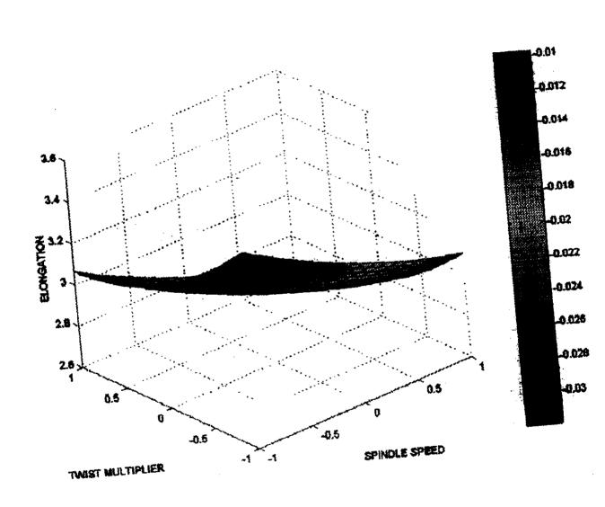
The effect of spindle speed and TM at a given traveler size of 10/O can be seen in the graph. It is observed that the yarn elongation value decreased gradually when the spindle speed is increased from 14000 to 16000 rpm. The change in yarn elongation was curvilinear when the TM is increased from 3.9 to 4.3. Thus for a given traveler number, the influence of spindle speed and TM was
