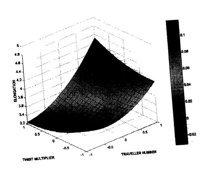
From the graph it can be observed that the yarn elongation falls with increase in TM from 3.9 to 4.3. On the other hand, yarn elongation gradually decreases with increase in traveler number from 10/O to 14/O. The effect of traveler number is much marked compared to TM.
