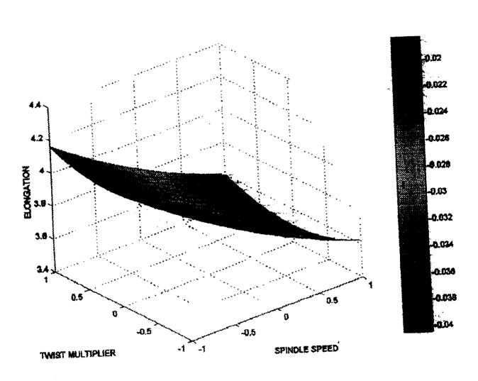
The effect of spindle speed and TM at a given traveler size of 12/O can be seen in the graph. It is observed that there is a drastical decrease in yarn elongation when spindle speed is increased from 14000 to 16000 rpm. The yarn elongation steadily increases with change in TM values from 3.9 to 4.3. Thus for the given traveler number the influence of spindle speed is more pronounced as
