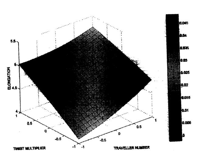
From the graph it can be observed that the yarn elongation increases sharply with increase in TM from 3.75 to 4.25. There is also a gradual increase in yarn elongation when the traveler number is varied from 6/O to 8/O. The change in yarn elongation was more marked in the case of varying traveler number
