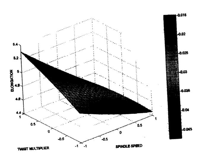
As per the graph at a given traveler number of 8/O, the yarn elongation abruptly decrease with increase in spindle speed from 14000 to 16000 rpm. The yarn elongation value increases almost linearly with increase in TM values between 3.75 and 4.25. The effect of spindle speed is much more pronounced
