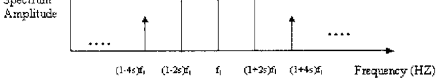
Fig. 2.5 Sideband frequencies around the fundamental line frequency
