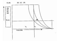
The ideal indicator diagram in fig ABCD illustrates the working of the compressor. Assuming, water jacket cooling bath and with no internal losses by friction or eddies, the graph is drawn. During the suction stroke AB, Volume  $(V_1)$  of air flows into the cylinder at atmospheric pressure  $(P_1)$  absolute and the work on the Piston is  $P_1V_1$ .
