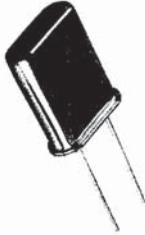
Fig 3.11 Piezoelectric Crystal Oscillator
