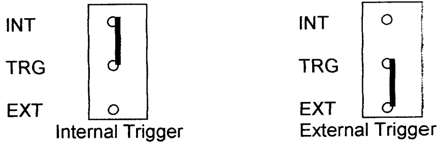
Fig 3.2 : Jumper settings for Trigger source selection.
