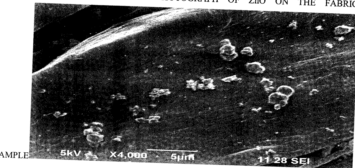
FIGURE 12 SHOWS THE SEM PHOTOGRAPH OF ZnO ON THE FABRIC
