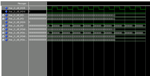
Figure 6.8: Waveform for the two-cycle MAC of operand size 64-bit
