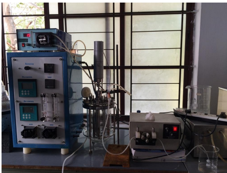
Figure 3.1 Experimental set-up of reactor for continuous dye removal
