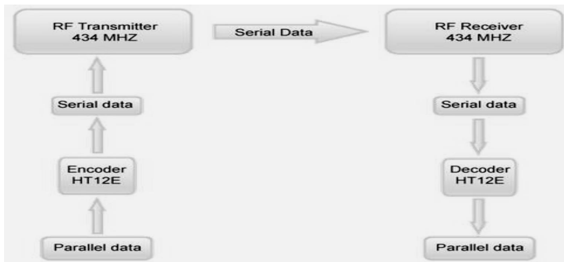
Figure 4.2.2 RF Transmitter-Receiver Block diagram [13]
