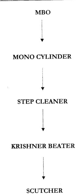
During the process 0.00158 hank was maintained. The trash and the cotton lap was found to be 0.48 % .Two separate lap one for each blend was chosen.
