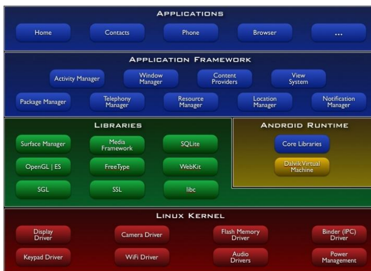
Fig 3.2 Architecture of Android development tool
