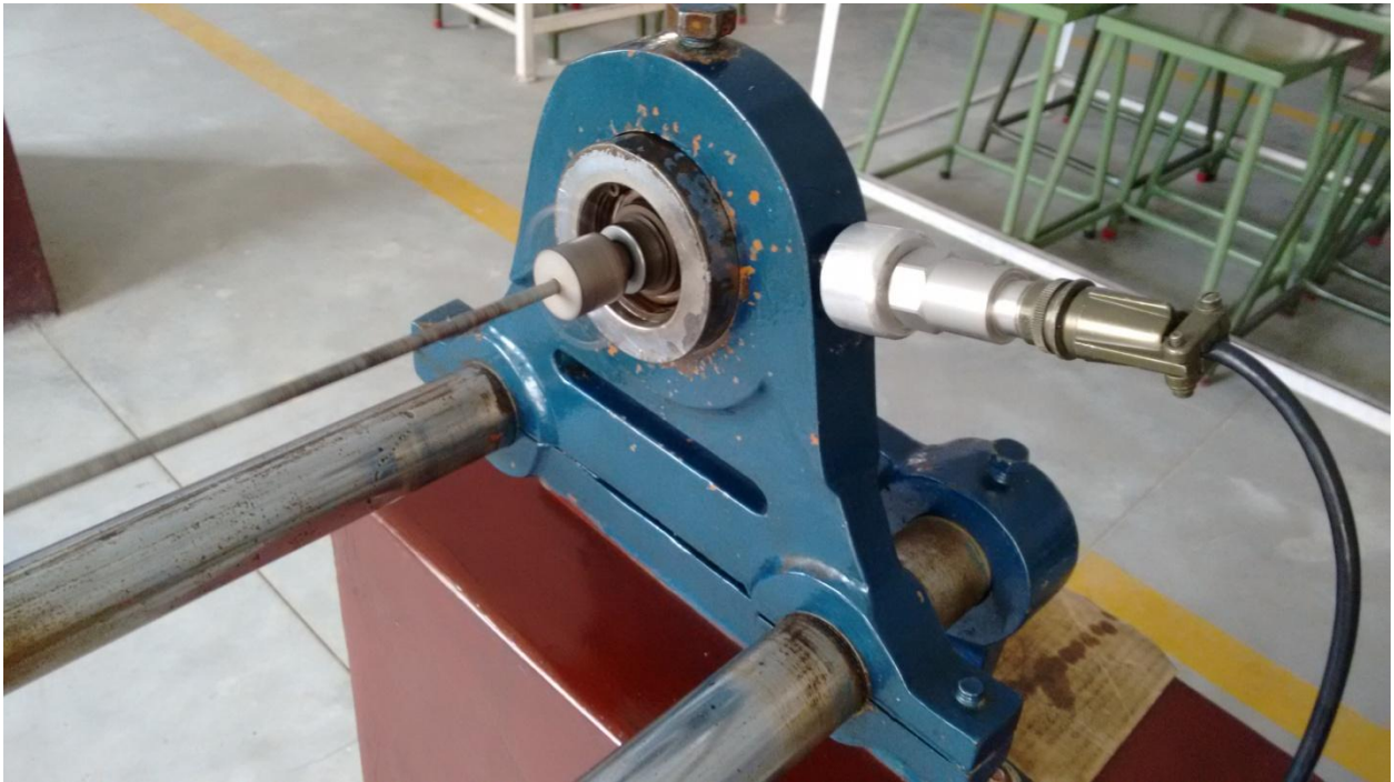
Fig.2.2 Accelerometer mounted on bearing
