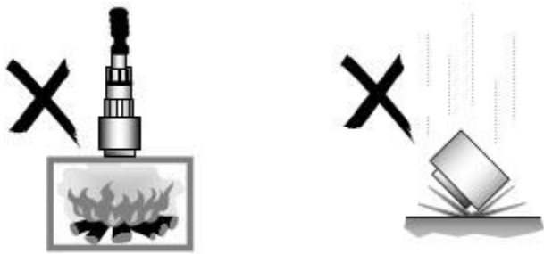
Fig.4.7 Improper removal of accelerometer
