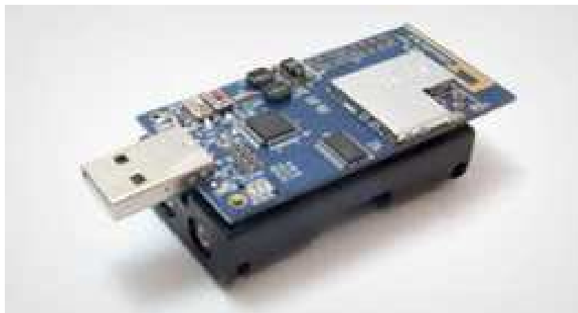
Figure3.3 CM5000 Sensor node
