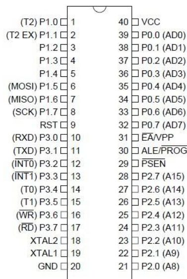
FIGURE 5.10: PIN DIAGRAM OF 89S52
