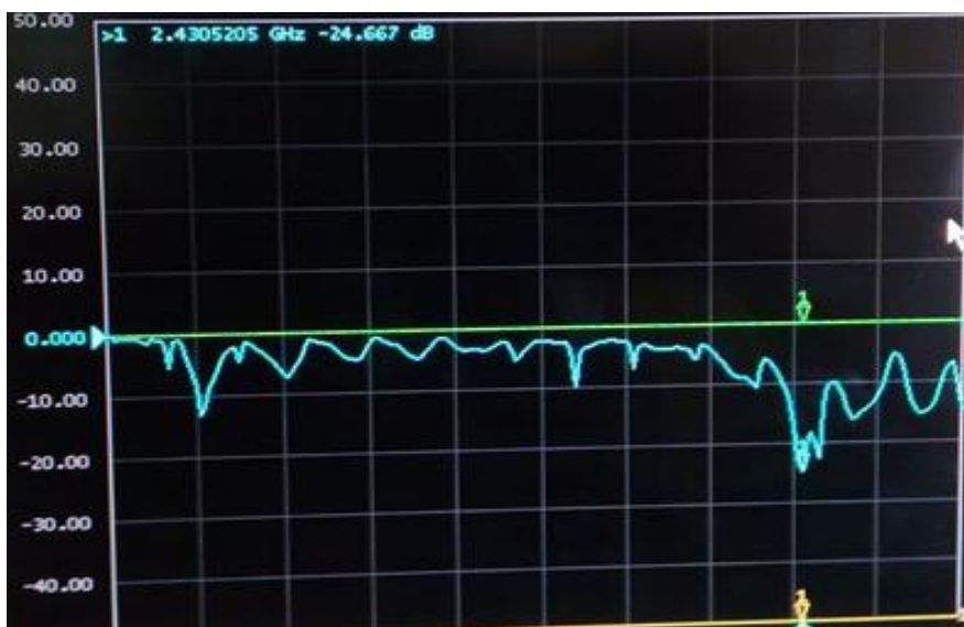
Figure 3.26 Fabricated result for return loss
