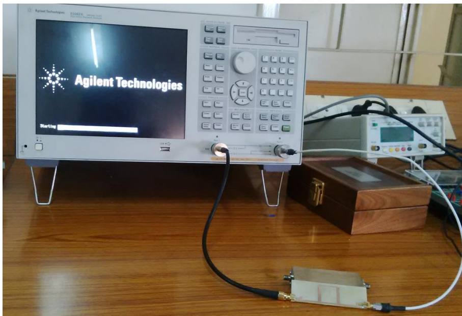
Figure 3.25 ENA Series Network Analyser E5062A conected with Triple band filter
