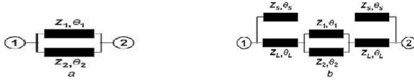
Figure 3.19 Configuration of (a) Basic filter section (b) Modified open stub filter section
