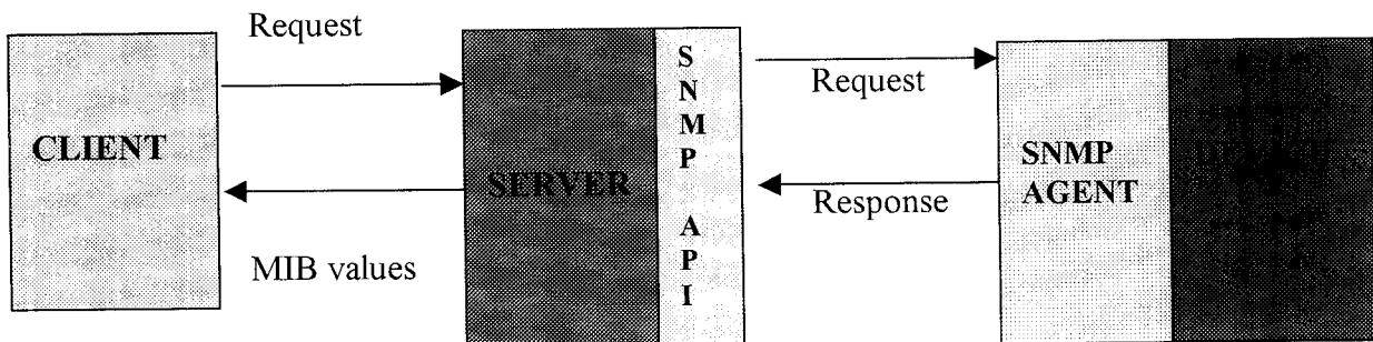
The client will connect to the server and the server connects to the device where its SNMP agent runs. The MIBs of the device will be read and values displayed to the client. The application will support any SNMP device. The architecture has the following features.
