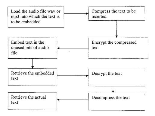
Once the text to be hidden is obtained from the user, it is compressed and then encrypted. While encrypting the text, a password (secret) key is obtained. Then the text is embedded into audio file. During retrieval the file is loaded, and the password should be given correctly to retrieve the text. But however the password doesn't match the user is not requested again to enter the password. But instead it is reported that the file contains some wrong text.
