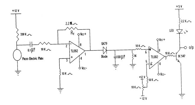
This accident announcement circuit is used to determine whether an accident has occurred or not. The accident is simulated by means of tapping the vibration sensor (piezo electric plate). Based on the intensity of vibration a signal will be sent to the micro controller depending upon the output of this circuit. It consists of the following sections.
