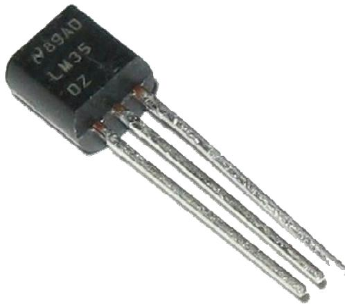
**Fig 4.2 89AD LM35 DZ Temperature Sensor**
