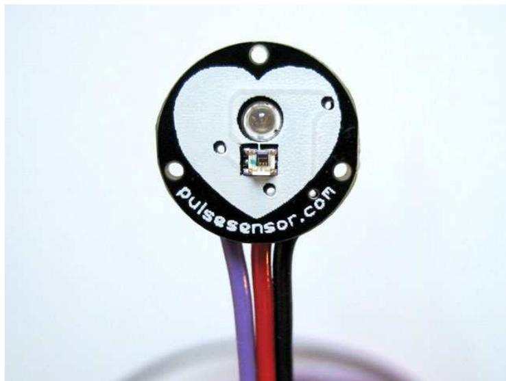
**Fig 4.3 Pulse rate Sensor**
